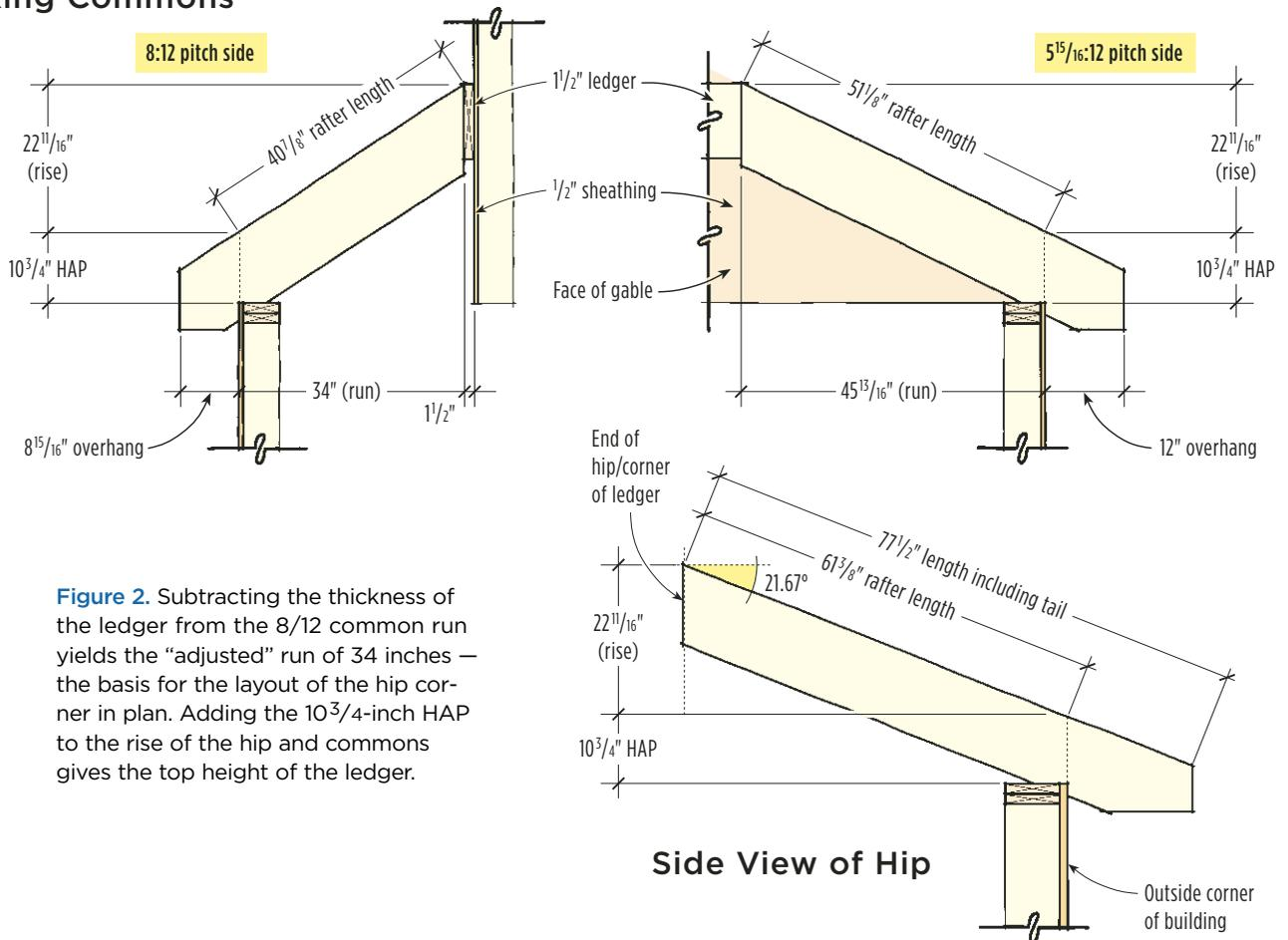
**Figure 2.** Subtracting the thickness of the ledger from the 8/12 common run yields the “adjusted” run of 34 inches — the basis for the layout of the hip corner in plan. Adding the 10 3/4-inch HAP to the rise of the hip and commons gives the top height of the ledger.
